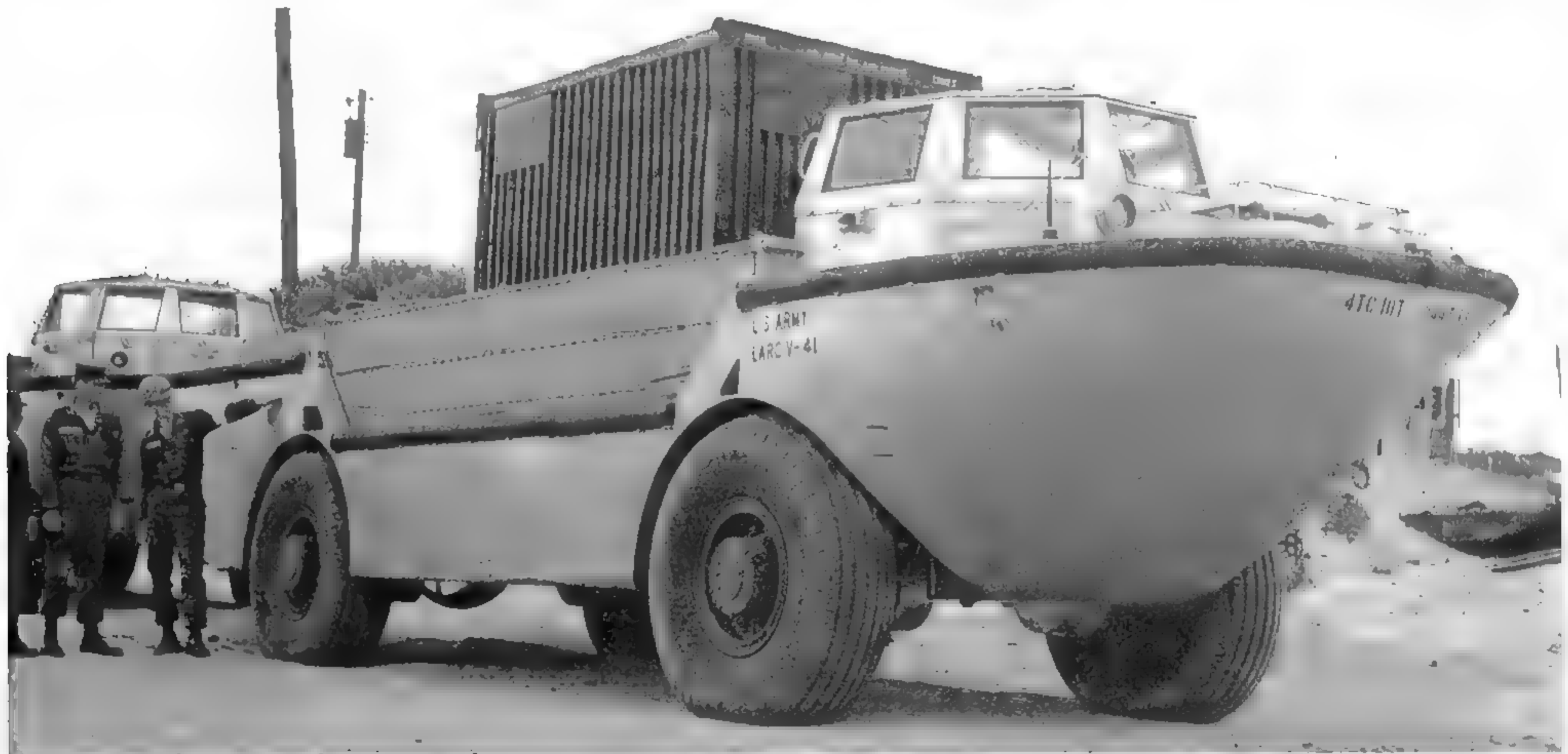
This is a LeTourneau-Westlinghouse LARC-V. It has been loaded with a CONEX container, and its side curtains have been raised in preparation for entering the water. (U.S. Army photo)
